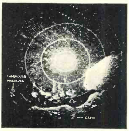
Fig. 11. PPI 'scope photographed a few hours before invasion of France. Plane has moved to within thirty-five miles of the coast, its position indicated by bright spot in center of 'scope. Invasion fleet (smaller blobs and grains) is clearly visible massed just off shore.
