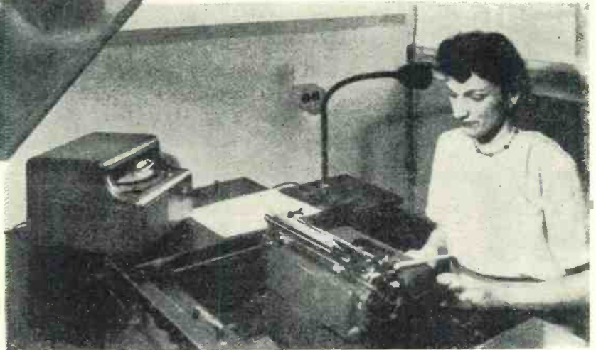
In playback operation, a loudspeaker is usually preferred. However, earphones can be used if desired.
